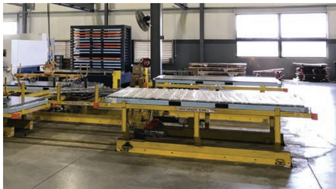
An empty staging table signals a fork truck driver to deliver material.
