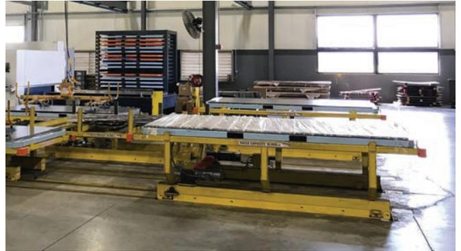
*An empty staging table signals a fork truck driver to deliver material.*
